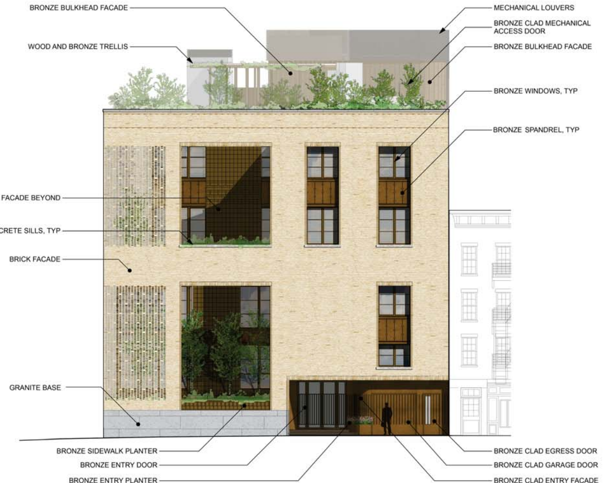
SOUTH ELEVATION (PERRY STREET) SCALE: 1/8" = 1'-0"
